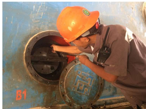
Gambar 5. Pengukuran nilai clereance bearing
